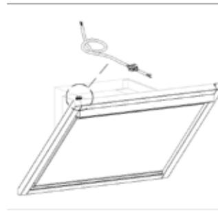
Electrical supply wire comes through the wall opening for the air evacuation.
